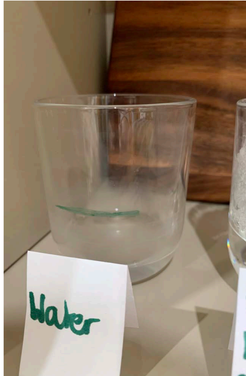
Water remains in the glass and limescale can be observed, leaving a cloudy film on the glass.
