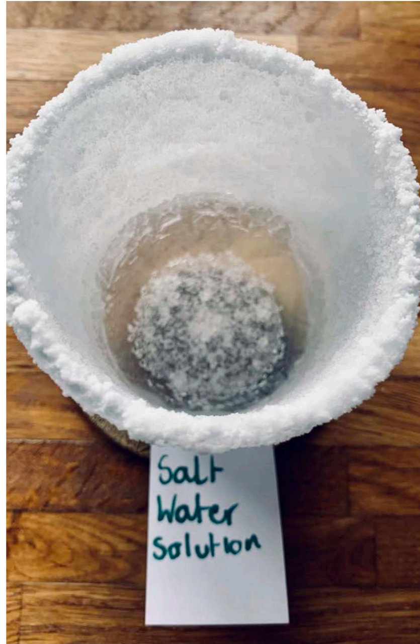
Salt is observed to have formed crystals that have completely covered the glass inside and out.
